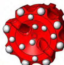
**CONCAVE****Applications / Anwendungen***Medium hard to hard formations, less abrasive, fractured formations, excellent control over hole deviation.*
